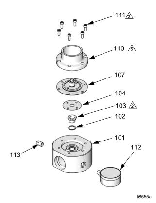
Fig. 3. Back Pressure Regulator Repair
