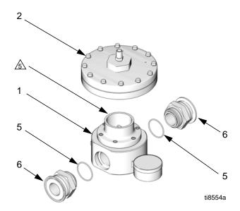
Fig. 2. Separate Diaphragm Housing from Back Pressure Regulator
