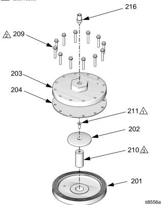
Fig. 4. Diaphragm Repair
